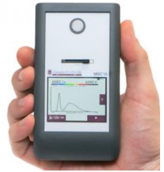
MSC15 for measurement of the illuminance, spectrum, color, and color rendering in the lighting industry
