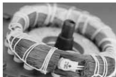
Fig. 42 Thermal switch incorporated in windings
