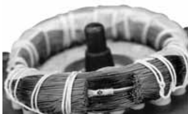
Fig. 40 PTC sensor incorporated in windings
